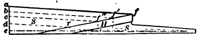
FIG. 57. Diagram illustrating Migration of a Fall due to a Hard Layer H , in the Midst of Soft Layers S and S , all dipping upstream
